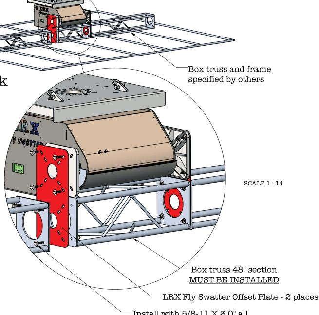
Install with 5/8-11 X 3.0" all thread grade 8 bolt assemblies
